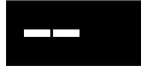
If the Valve's setpoint is changed when the Thermostat is OFF, the Valve displays two white dashes on a black background
